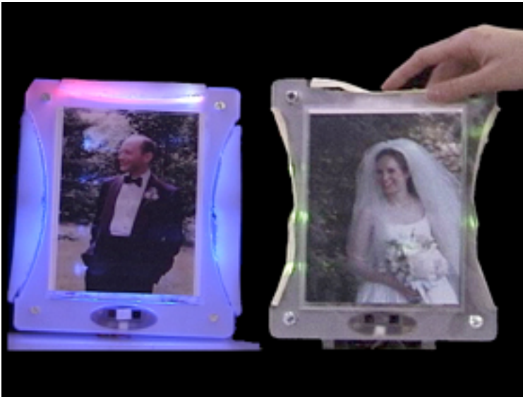
Fig. 2- LumiTouch used light and vibrotactile feedback with picture frames to explore presence between remote users.
