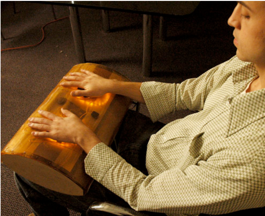
Figure 19 – Impulse by Gilad Lotan and Christian Croft transmits heartbeats via haptics over local network to another user
